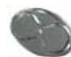
0428-3 Couvre serrure porte de soute, pick-up cabine unique Side compartment key cover, pick-up single cabin • Type 2 -08/66
