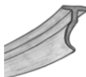
0724 Joint entre cloison pare-feu et moteur, vertical Rubber around engine, vertical, between firewall and engine
